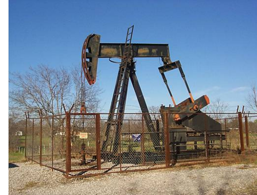
Stripper well; Source: J. Veil, Argonne National Laboratory
